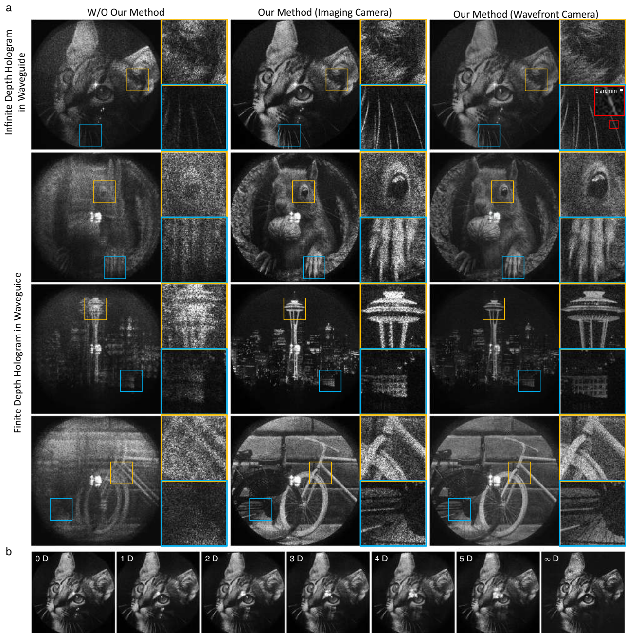
Fig. 4 | Experimental results of waveguide holography. a The first column illustrates the results captured without our method while the second and third columns illustrate the result with holograms generated using our model, captured with imaging camera and wavefront camera respectively. Finite depth images are displayed at 3 diopter (D) from the user's pupil. The yellow/blue insets correspond to 1.3 degree of field of view and red inset corresponds to 10 arcmin. Limited fill
